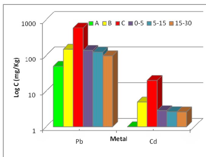
Figure 3. Median soil concentrations of Pb and Cd at three depths in comparison to the Dutch classification scheme levels (Verner *et al.*, 1996).
